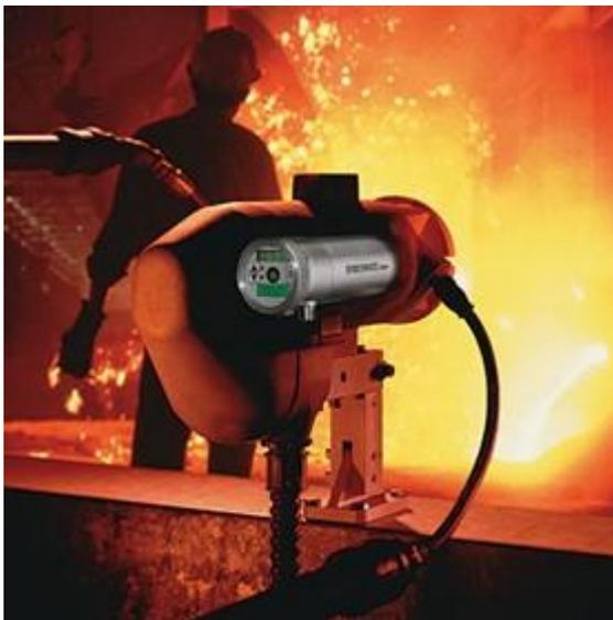
In the iron and steel industry, temperature measurement helps to ensure that the correct heating or cooling is applied. Benefits in getting this right include better quality, increased productivity, enhanced safety, reduced downtime, easy data recording and reduced energy costs.
