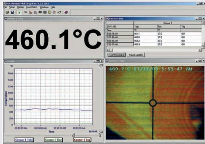
Plot the temperature values of an MM sensor with a video image. High and low alarms are shown, making it easy to identify out-of-range conditions. DataTemp Multidrop software makes it easy to remotely configure smart MM sensors from the safety of the control room.
